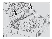
2 Open the transport guide while holding the knob (A).
